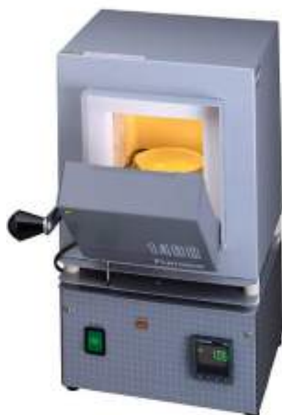
Muffle furnace: It is used to burn precipitates over 1000^\circ\text{C} temperature.
