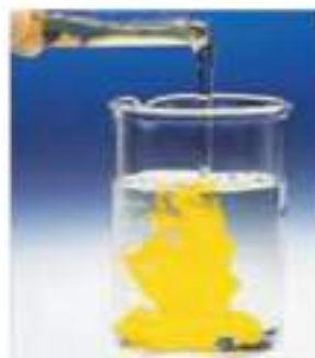
Addition of chemical reagent to the sample solution and formation of the precipitate
