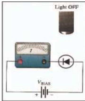
Figure (29) The photosensitive (PN) diode before the light is incident on it. The current is not flow in its circuit, notice the ammeter (The current is zero).
