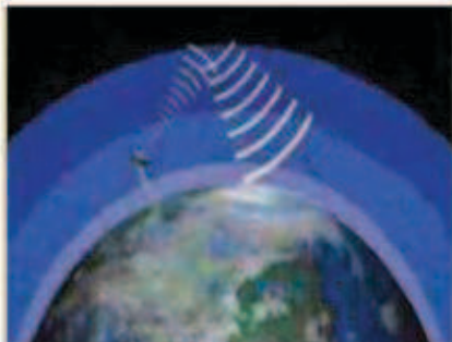
Figure 6 : Every layer in the atmosphere has an advantage for humans. The Ionsphere, for example, reflects the radio waves which are transmitted from a certain centre to the earth. This can allow the transmission to the far distances.
