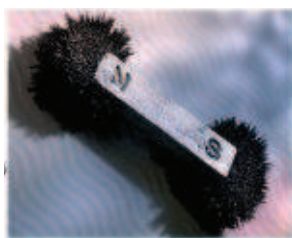
Figure 7a explains accumulating the iron filling with high concentration at the magnet poles.
