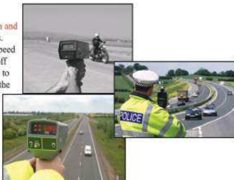
Figure 11.4 Police officers use radar to detect cars going faster than the speed limit.
