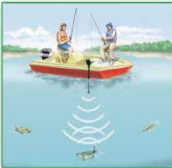
Figure 6 A fish finder sends ultrasonic waves down into the water. The time it takes for the echo to return helps determine the location of the fish.
