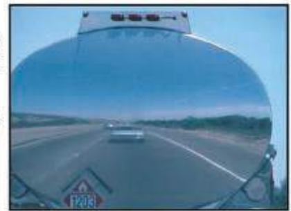
Figure 8.3 The shiny and curvy back surface of a tanker acting as a convex mirror
