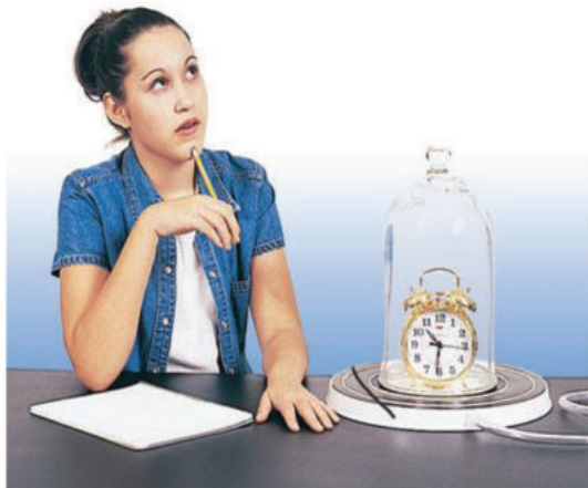
Figure 3 Tubing is connected to a pump that is removing air from the jar. As the air is removed, the ringing alarm clock sounds quieter and quieter.
