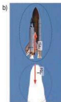
Figure 11 The rocket exerts an action force on the gas and the gas exerts an equal and opposite force upon the rocket. Thus, the rocket moves forwards
