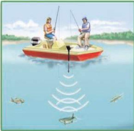
Figure 6 A fish finder sends ultrasonic waves down into the water. The time it takes for the echo to return helps determine the location of the fish.
