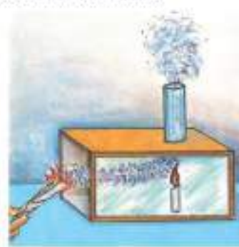
Figure 7.8 Demonstration of convection currents in air.
