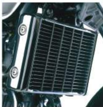
Car and motorcycle radiators are painted black to radiate away heat as quickly as possible.
