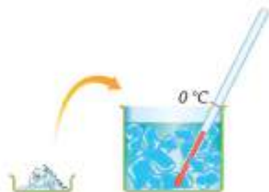
Figure 8.16 Adding salt decreases the freezing point of water.
