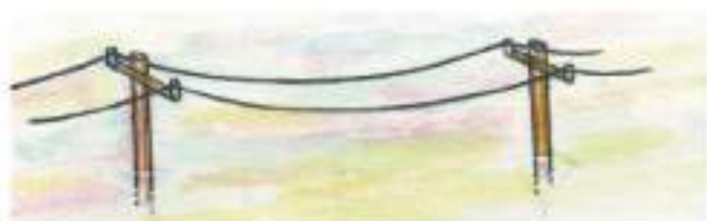
Telephone cables expand in summer.
