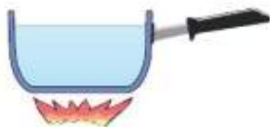
Figure 7.2 Plastic handles prevent heat conduction
