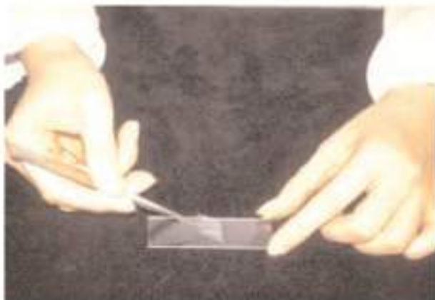
3. Lower the cover glass slowly to avoid air pockets, pull the tweezers out.
