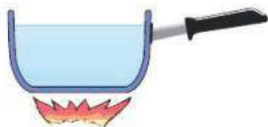
Figure 7.2 Plastic handles prevent heat conduction
